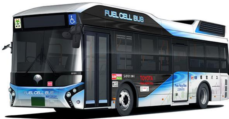
FC Bus with two Mirai's FC systems sold to the Tokyo Metropolitan Government, February, 2017
